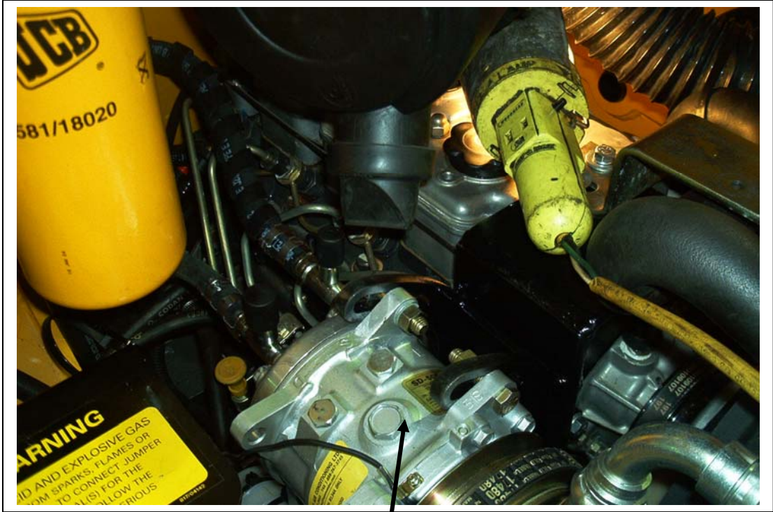
Compressor in place
